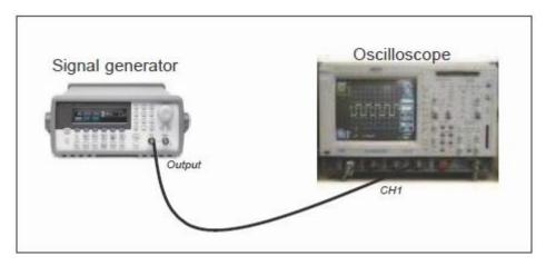
Set the DC mode coupling on the oscilloscope.
