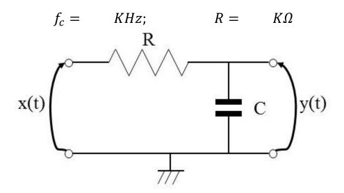
Measure the amplitude and phase characteristics of the signals and the complete the following table, remember that:
